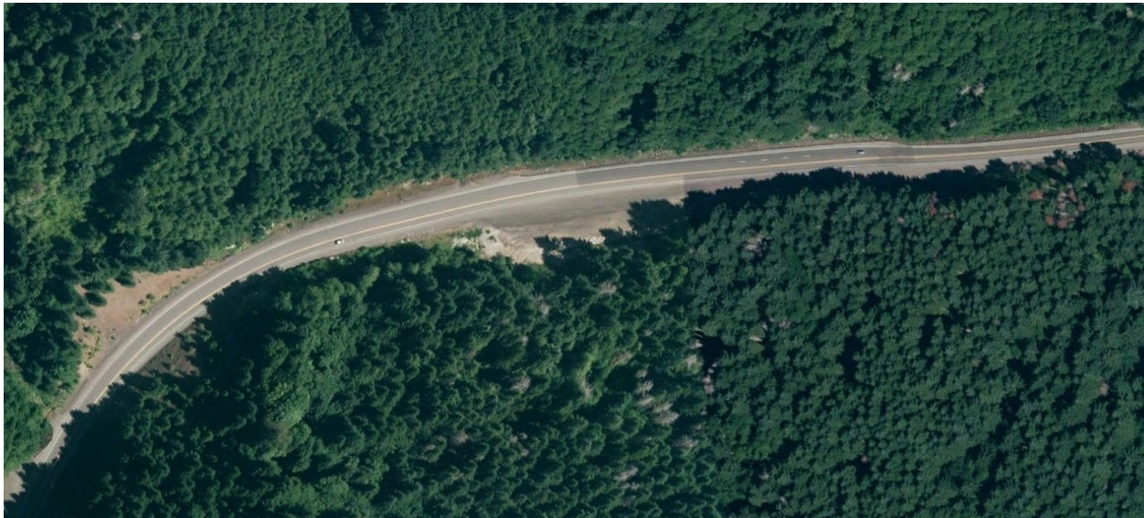
Exhibit 4. Illustration of Existing Passing Lane with Striping According to Latest MUTCD Guidance (Photo Source: Google Earth)
