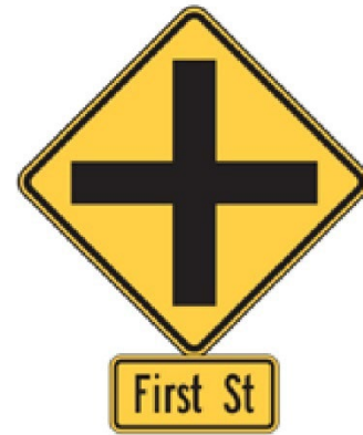
Photo/Image Credit: FHWA Manual on Uniform Traffic Control Devices (W2-1 with W16-8P supplemental plaque)
